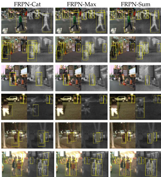
Fig. 5. Qualitative comparison of multispectral pedestrian detection results of FRPN-Cat, FRPN-Max, and FRPN-Sum. Note that yellow bounded boxes show pedestrian detections.
