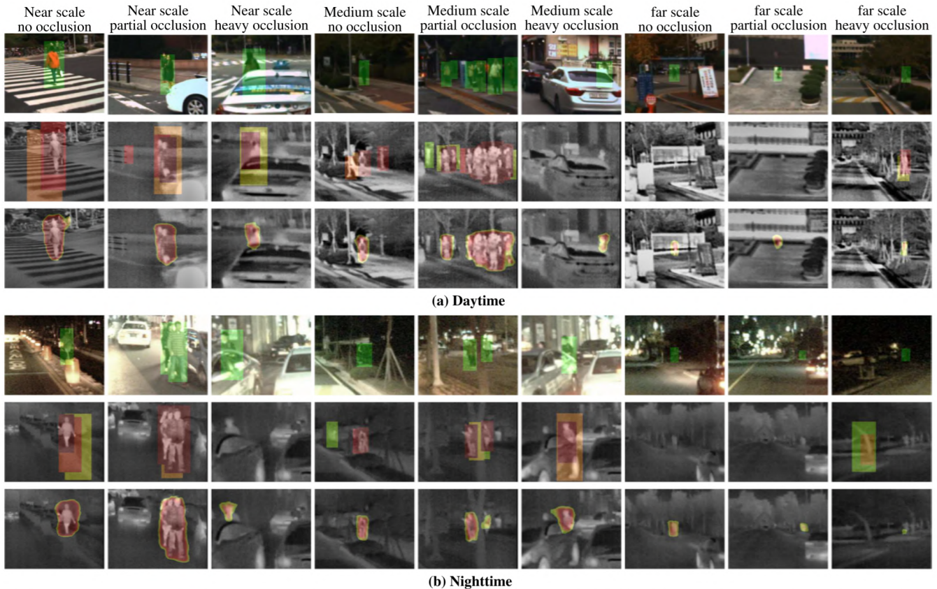
Fig. 6. Qualitative comparison of multispectral pedestrian detection results of RPN-HMFFN-640 and HMFFN-640 in the KAIST testing dataset. First row shows the ground truth (displaying using the visible channel) and the others show detection results of RPN-HMFFN-640 and HMFFN-640 respectively (displaying using the infrared channel). Note that the green regions represent ground-truth annotation masks which are generated based on manually labeled bounding boxes, and the detected pedestrian targets are visualized using the heat map representation with a 0.5 threshold. Best viewed in color. (For interpretation of the references to color in this figure legend, the reader is referred to the web version of this article.)
