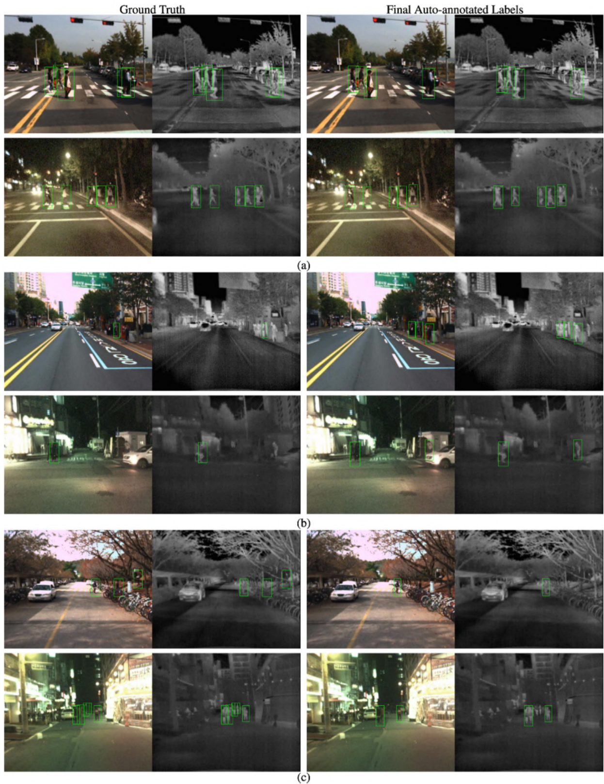
Fig. 9. Examples of final auto-annotated positive labels and ground truth. (a) Our auto-annotation results are comparable with ground truth; (b) our results are better than the ground truth annotations (some true positives which are missed by human observers are correctly identified by our auto-annotation approach); (c) our results are not satisfactory (some insignificant pedestrian samples are not correctly annotated). Note green bounding boxes show positive labels. (For interpretation of the references to color in this figure legend, the reader is referred to the web version of this article.)
