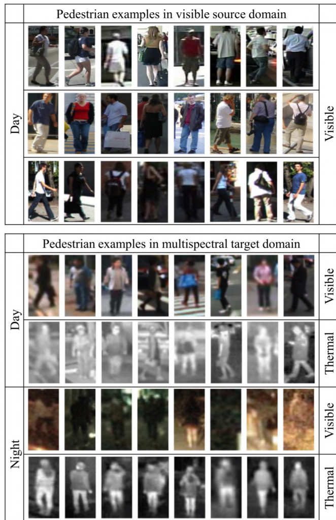
Fig. 2. Examples of pedestrians in the visible daytime source domain [8,37,39] and the multispectral (visible and thermal) target domain [13]. It is noted pedestrian instances exhibit significantly different human-related characteristics in the visible and thermal channels captured during daytime and nighttime.
